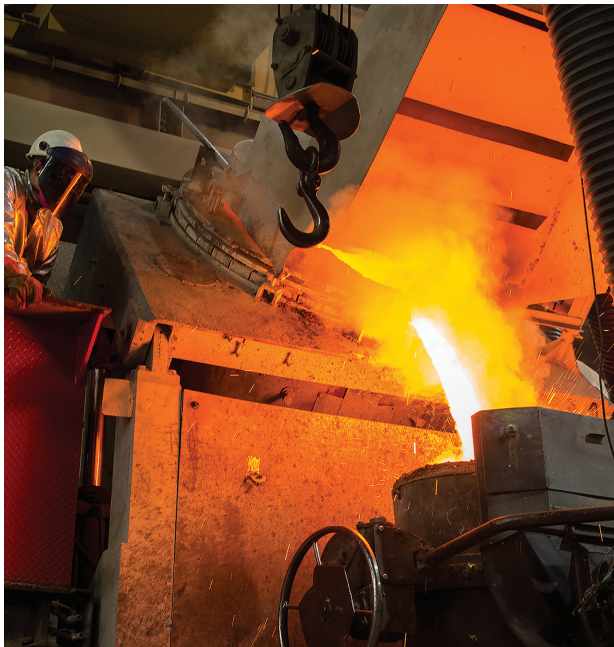
Standard bronze pour from furnace to ladle in our foundry for EXCEL parts, located in Pekin, Illinois, USA
