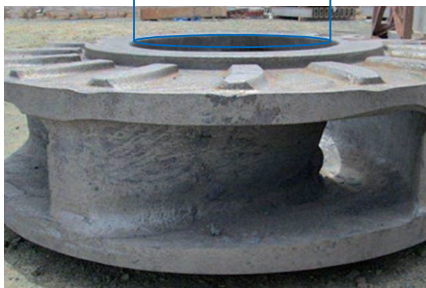
millMAX pump impeller eye is protected from recirculation wear by the wear ring
