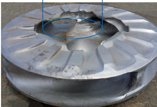
Competitor's pump impeller eye is enlarged and deformed, indicating suction-side recirculation
