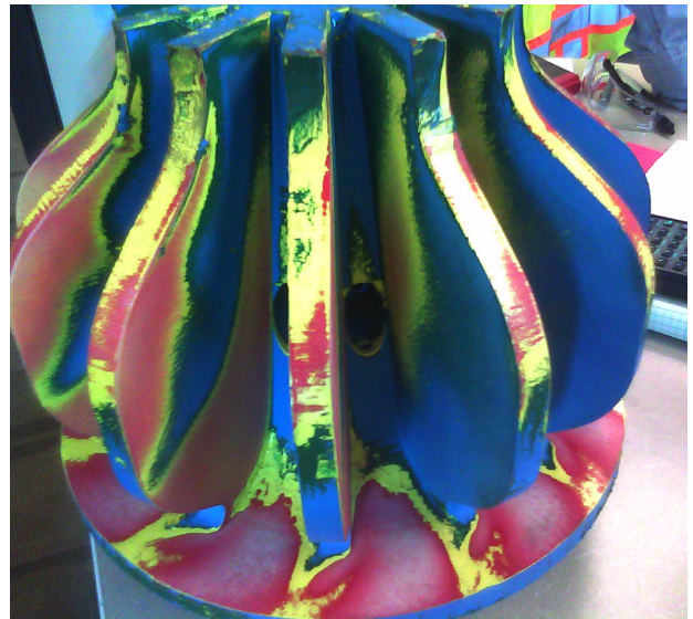
Wide flow jets produced by the nextSTEP rotor and the cross pattern from the patented slotted nextSTEP stator increase the chances of flotation
