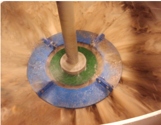
Wide flow jets produced by the nextSTEP rotor and the cross pattern from the patented slotted nextSTEP stator increase the chances of flotation
