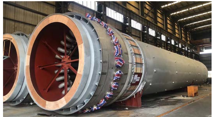
Completed rotary cooler awaiting transport to a new lithium refinery
