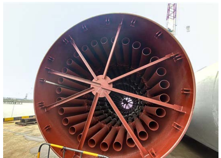
Internal air pipes
