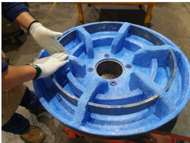
An example of FLSmidth WEAR MAX ® applied to surface of a HFC Feed Distributor
