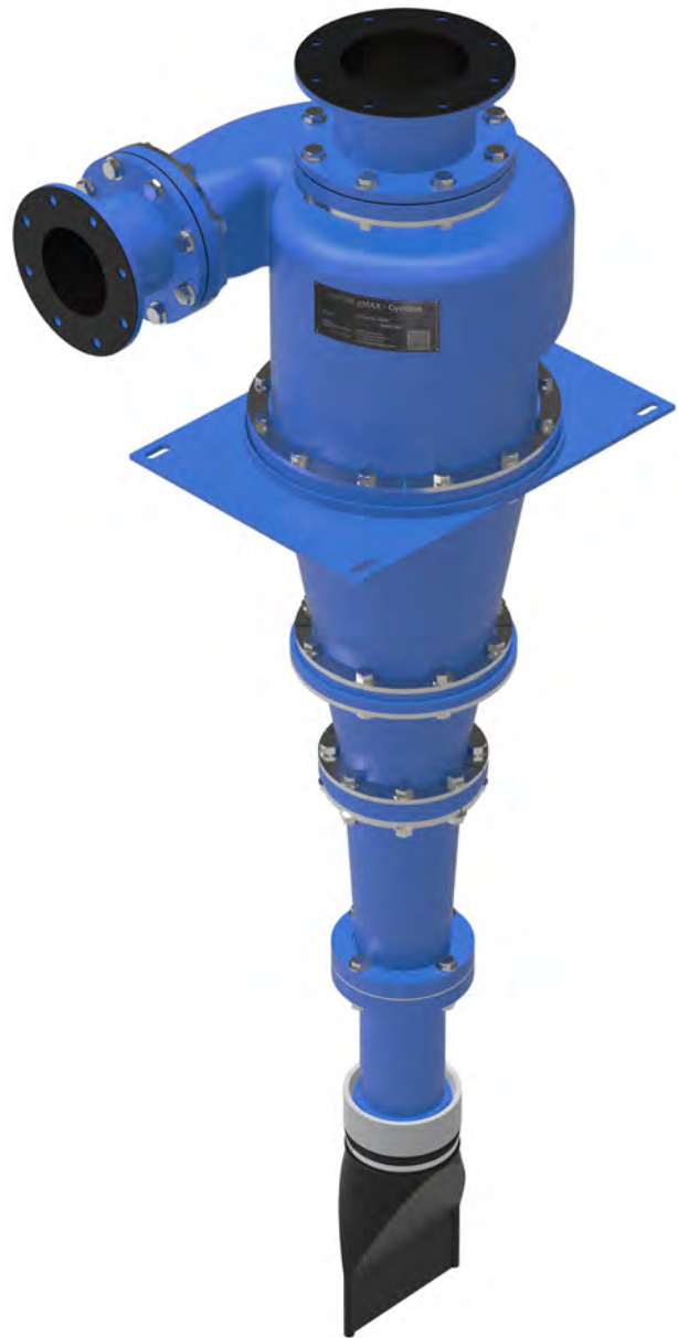
CycloStack boot installed on apex of cyclone to control the moisture in the coarse sand discharge
