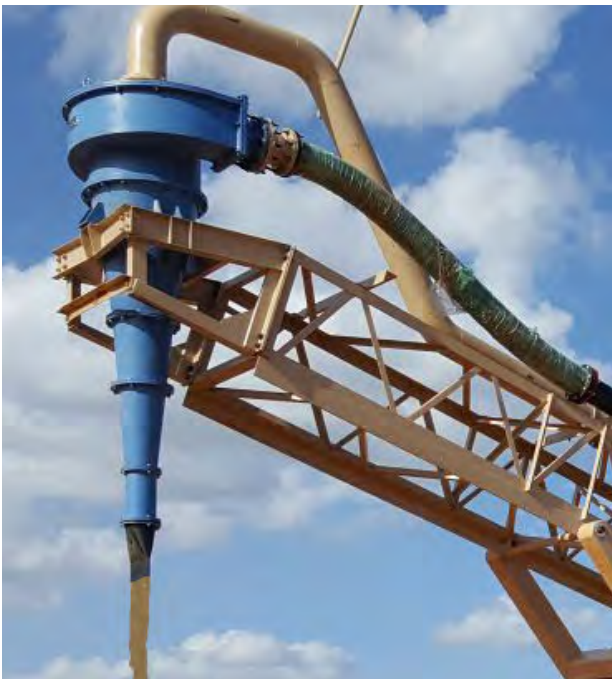
Solids discharging through CycloStack
